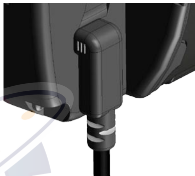
GXM 30 Antenna Plugged In
